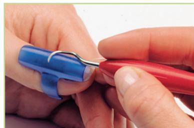
On either side of the LM-RondoPlus™ there are LM-Fingo™ test sticks. Sharpness can be tested both with Fingo mounted on the LM-RondoPlus™ or your finger. The Fingo is made of an acrylic plastic and is sized to fit all users.
