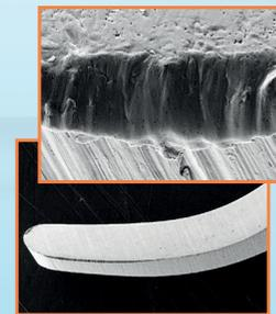
Cutting edge of a typical non-coated curette and the magnification of the edge after the test.
