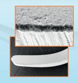
Cutting edge of the LM Sharp Diamond<sup>™</sup> curette and the magnification of the edge after the test.
